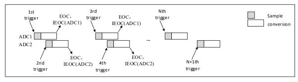
Figure 12-10 Alternate trigger: injected channel group of each ADC
