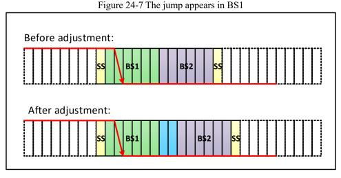
As shown in Figure 24-7, the SJW is 2, and the bus level transition is detected in the time period 1, then the length of the time period 1 needs to be extended, and the maximum SJW is extended, thereby delaying the position of the sampling point.
