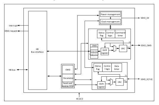
Figure 28-1 SDIO structure diagram
