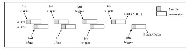
7) Regular simultaneous mode + Injected simultaneous mode
