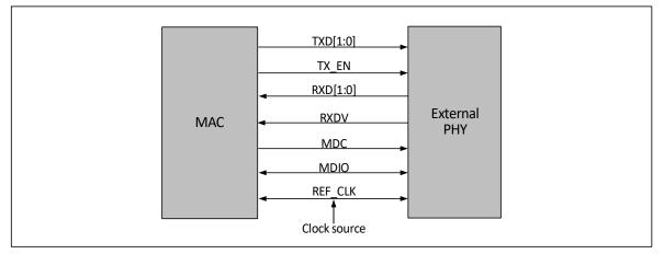
*Note: The Ethernet transceiver needs to input the externally provided REF\_CLK 50MHz clock frequency from the RXC pin.*
