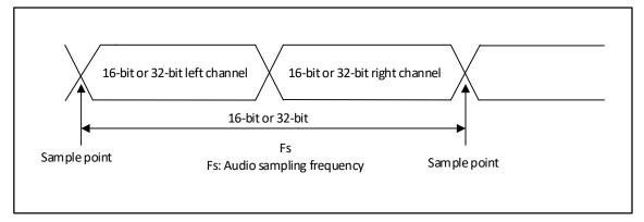
Figure 20-15 Audio sampling frequency definition
