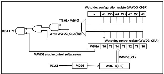
Figure 8-1 Window Watchdog block diagram
