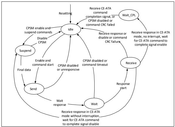
Figure 28-2 Command path state machine
