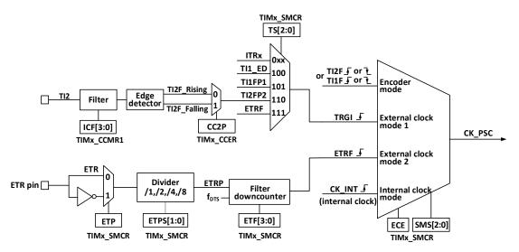
Figure 14-2 CK\_PSC source block diagram of advanced-control timer
