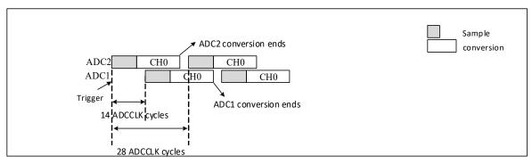
*Note: 1. The sampling time should be less than 14 ADC clock cycles, to avoid an overlap with the next conversion;*
