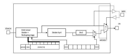
The clock source of I2SxCLK in the figure is the system clock (i.e., the HSI, HSE, or PLL that drives the HB clock). I2SxCLK can come from SYSCLK, or the PLL3 VCO (2xPLL3CLK) clock, which can be selected by the I2S2SRC and I2S3SRC bits in the RCC\_CFGR2 register. Audio can be sampled at 96KHz, 48KHz, 44.1KHz, 32KHz, 22.05KHz, 16KHz, 11.025KHz, or 8KHz (Or any value within this range). To obtain the desired frequency, set the linear divider according to the following formula:
