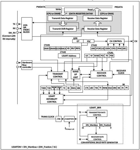
Figure 18-1 USART block diagram
