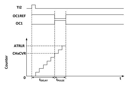
Figure 14-5 Single pulse generation
