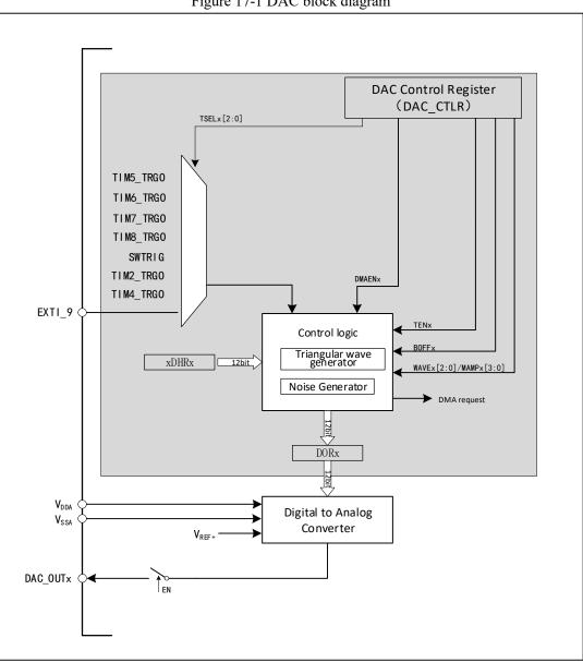
Figure 17-1 DAC block diagram
