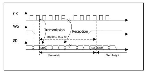
Figure 20-4 Philips protocol waveform (16/32 full precision, CPOL=0)
