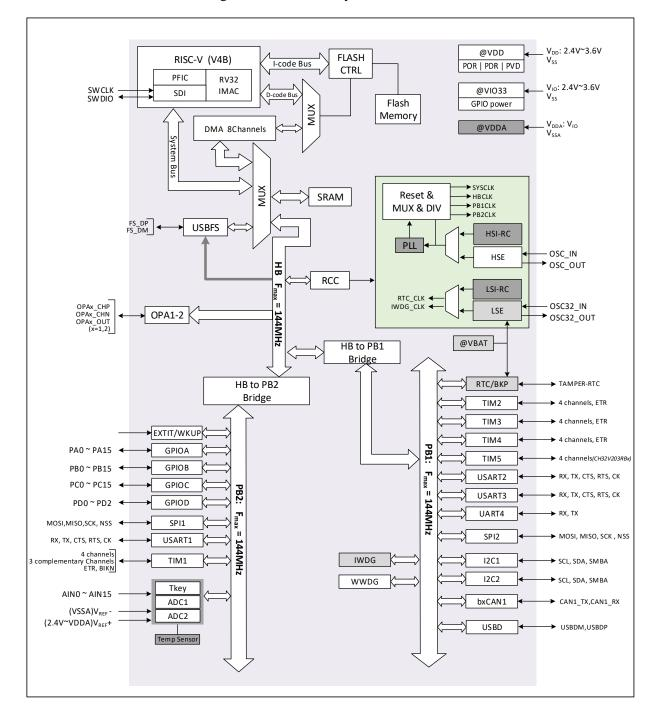
Figure 1-4 CH32V203 system architecture
