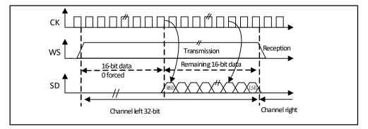
During the I2S configuration stage, if you choose to extend the 16-bit data to a 32-channel frame, you only need to access the DATAR register once. At this point, the high half word (16-bit MSB) after extending to 32 bits is set to 0x0000 by hardware.
