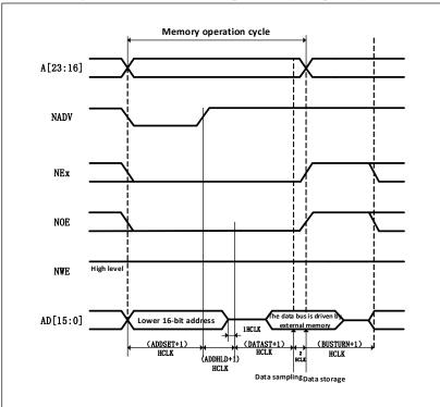
Figure 26-7 Mode B read operation (multiplexed)
