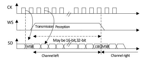
Figure 20-7 MSB aligned 16-bit or 32-bit full precision (CPOL = 0)
