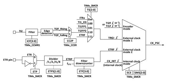
Figure 15-2 Block diagram of general-purpose timer source
