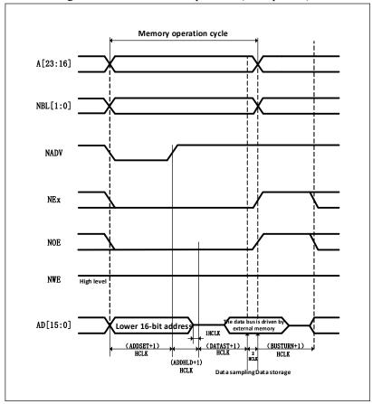
Figure 26-9 Mode C read operation (Multiplexed)
