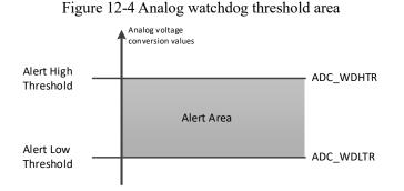
Configure the AWDSGL, AWDEN, JAWDEN and AWDCH[4:0] bits in the ADC\_CTLR1 register to select the channel for analog watchdog vigilance. The specific relationship is shown in the following table:
