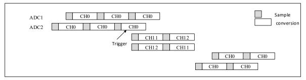
Note: When the ADC clock prescaler is set to 4, the sampling interval is 8 ADC clock cycles followed by 6 ADC clock cycles, instead of 7 ADC clock cycles followed by 7 ADC clock cycles.
