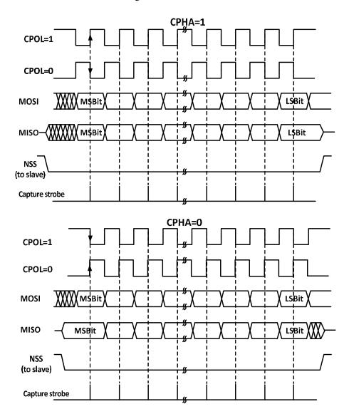
Figure 20-2 SPI model
