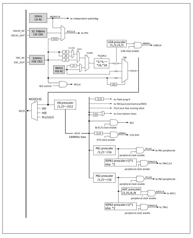
Figure 3-5 CH32FV208 clock tree structure
