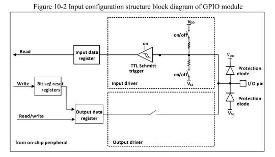
When the IO port is configured as input mode, the output driver is disconnected, the input pull-up and pulldown are optional, and the alternate function and analog input are not connected. The data on each IO port is sampled to the input data register at each PB2 clock, and the corresponding bit of the input data register is read to obtain the level state of the corresponding pin.
