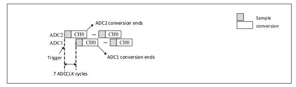
Figure 12-8 Fast interleaved mode on 1 channel in continuous conversion mode
