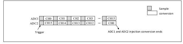
*Note: 1. Do not convert the same channel on ADC1 and ADC2;*
