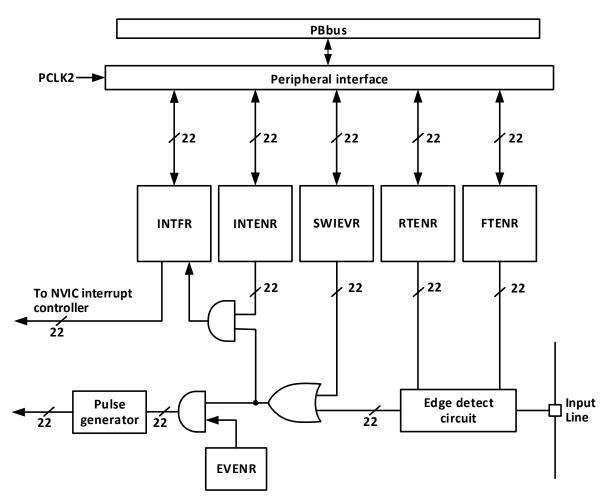
Figure 9-1 External interrupt (EXTI) interface block diagram
