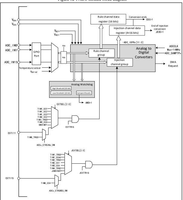
Figure 12-1 ADC module block diagram
