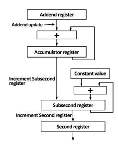
Figure 27-10 Process for updating time using fine correction
