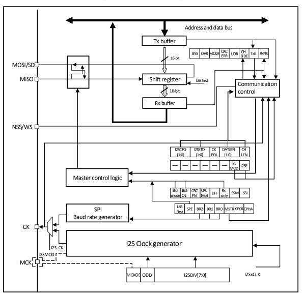
Figure 20-3 I2S structure diagram
