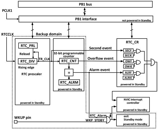
As shown in Figure 6-1, the RTC module is mainly composed of 3 parts: PB1 bus interface, prescaler and
