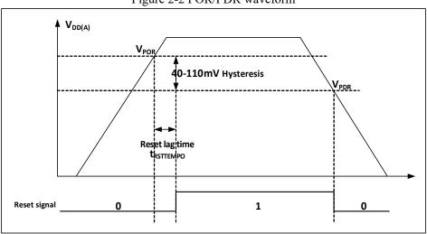
Figure 2-2 POR/PDR waveform
