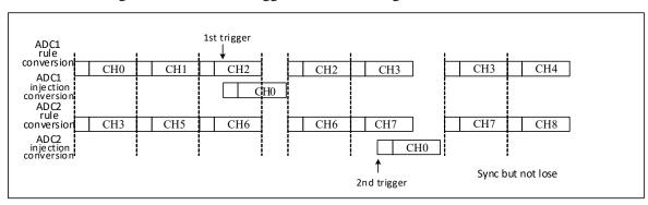
Figure 12-12 Alternate trigger conversion in regular simultaneous mode
