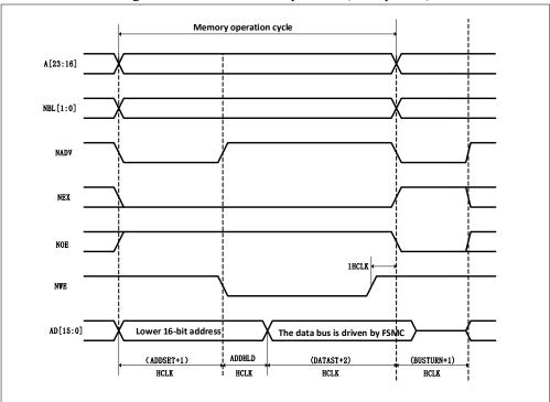
Figure 26-4 Mode 1 write operation (Multiplexed)
