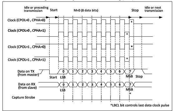
Figure 18-2 Example of USART clock timing (M=0)
