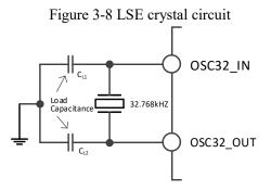
• External low-speed clock source (LSE bypass): In this mode, an external clock source is directly provided to the OSC32\_IN pin, and the OSC32\_OUT pin is suspended. The application program needs to set the LSEBYP bit when the LSEON bit is 0, to enable the LSE bypass, and then set the LSEON bit.
