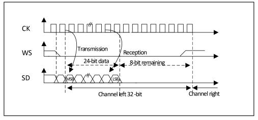
This mode requires 2 read or write operations to the SPI\_DATAR register. In transmit mode: if you need to send 0x8EAA33 (24 bits):
