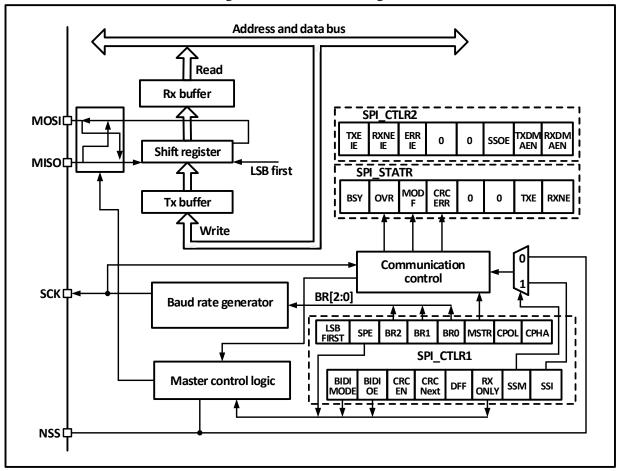
Figure 20-1 SPI structure diagram
