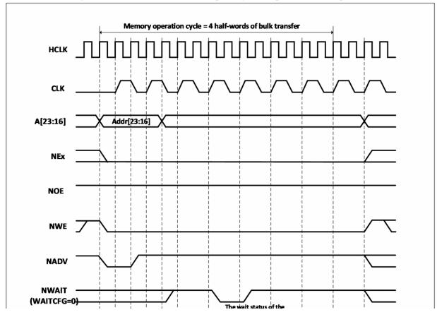
Figure 26-14 Synchronous bus multiplexing write operations (Multiplexed)
