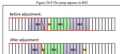
As shown in Figure 24-8, the SJW is 2, and the bus level transition is detected in the time period 2, so it is necessary to reduce the length of the time period 2 and reduce the SJW at the maximum, so as to advance the position of the sampling point.
