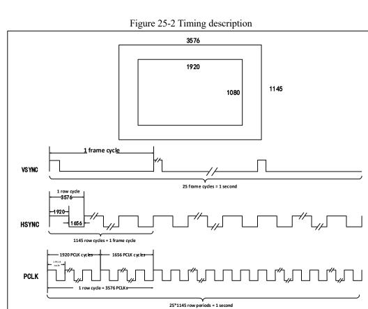
PCLK is the transmission time of a pixel, so HSYNC is 3576 times more than PCLK. Among the 3576 pixels, only 1920 pixels are valid, and the sensor does not transmit data during the remaining 1656 pixels. VSYNC is a frame synchronization signal, so the VSYNC time is 3576\*1145 times of PCLK. Similarly, the sensor is transmitting data only during the 1920\*1080 effective pixel time. If the sensor is transmitting JPEG compressed data, the HSYNC signal may not be needed.
