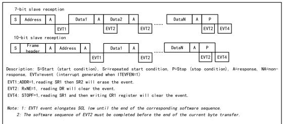
The master device will generate a stop condition after the last data byte is transferred. When the I2C module detects a stop event, it will set the STOPF bit, and if the ITEVFEN bit is set, it will also generate an interrupt. The user needs to read the status register (R16\_I2Cx\_STAR1) and then write the control register (e.g. reset control word SWRST) to clear it. (See EVT4 in the figure above).
