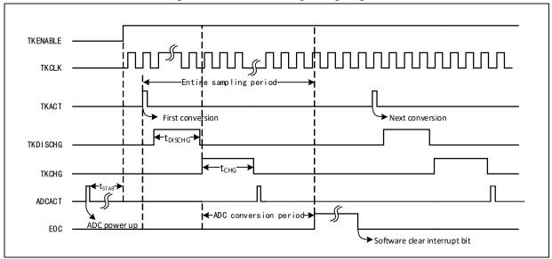
Figure 13-1 TKEY working timing diagram
