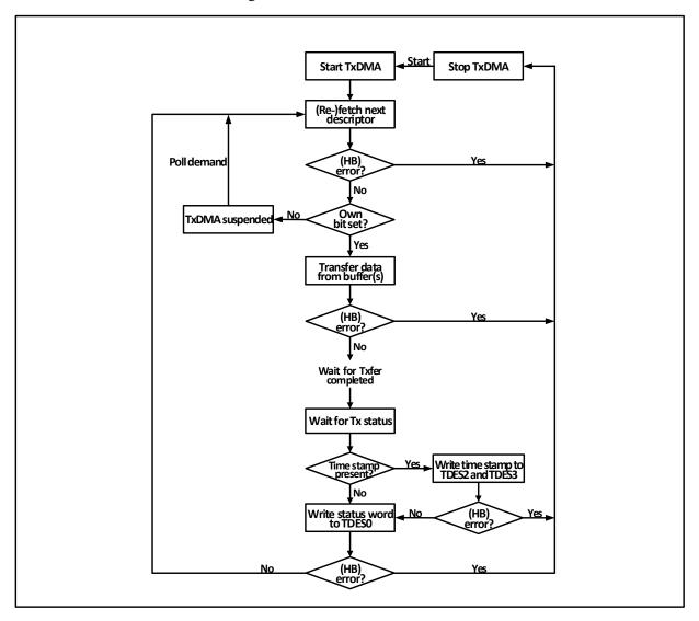
Figure 27-11 Process of transmission
