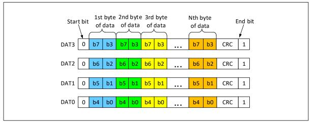
Figure 28-11 SD card single bus data transfer in a 512-bit word format
