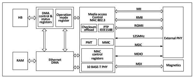
In addition, the Ethernet transceiver also supports the IEEE1588 Precision Time Protocol (PTP) to provide precise time data for microcontroller systems or off-chip.
