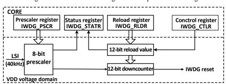
Figure 7-1 Structure block diagram of Independent Watchdog
